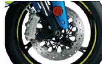
Front brake system with Brembo
